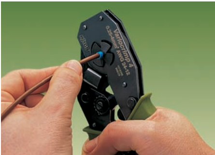
Squeeze handles until ratchet mechanism is released.
